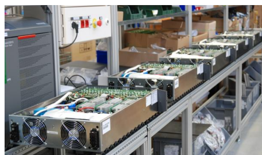
Power Module assembling line Socomec manufacturing facility (Italy) Quality management system ISO 9001:2008
